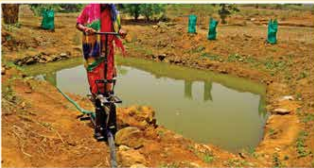
Sarendri Patra is lifting water through Treadle Pump to irrigate her family farm at Uppergodi village of Lamtaguda G.P.
